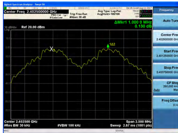
(1Mbps) Channel Separation plot on channel 39-40
