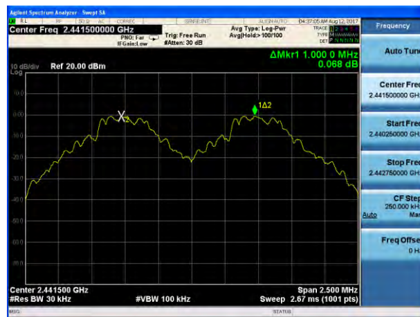
(1Mbps) Channel Separation plot on channel 77-78
