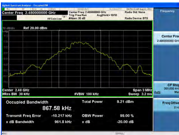
20dB Bandwidth plot on channel 78 (1Mbps)
