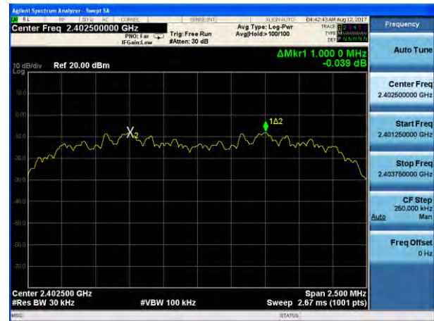
(2Mbps) Channel Separation plot on channel 39-40
