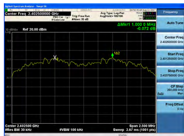
(2Mbps) Channel Separation plot on channel 77-78
