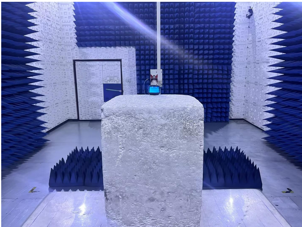
RADIATED EMISSION TEST SETUP ABOVE 1GHz
