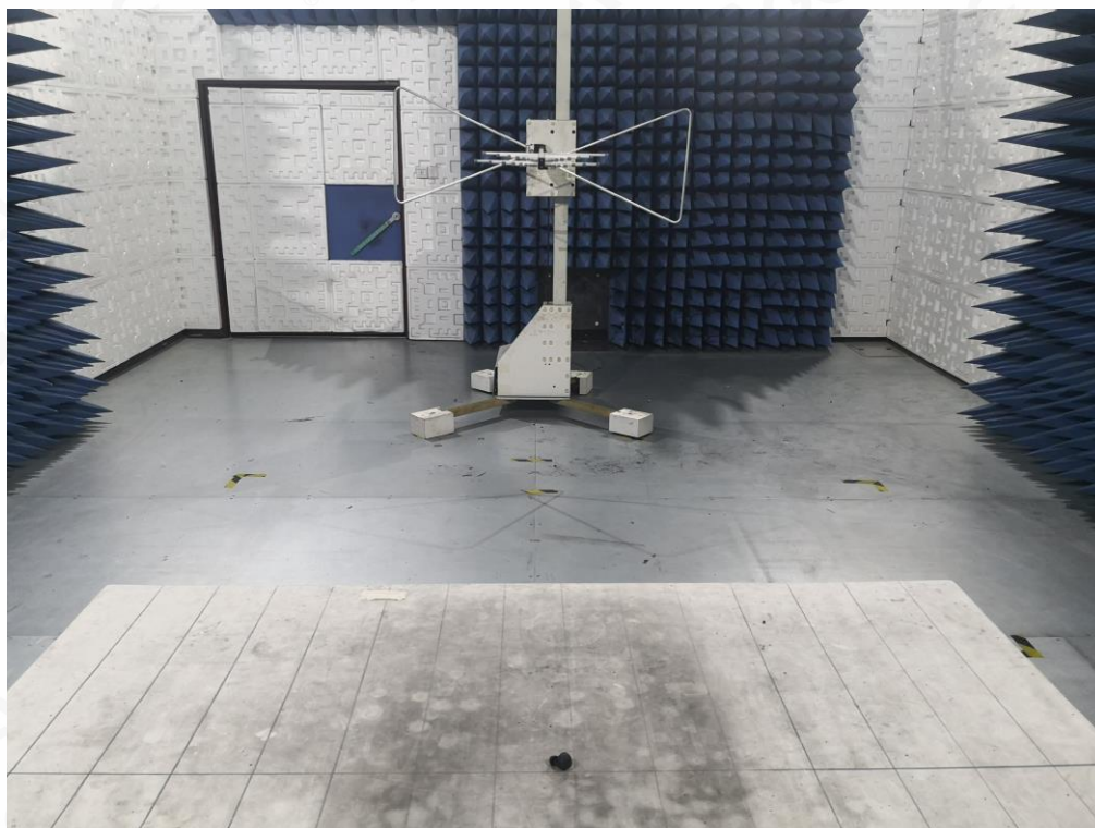
RADIATED EMISSION TEST SETUP ABOVE 1GHZ
