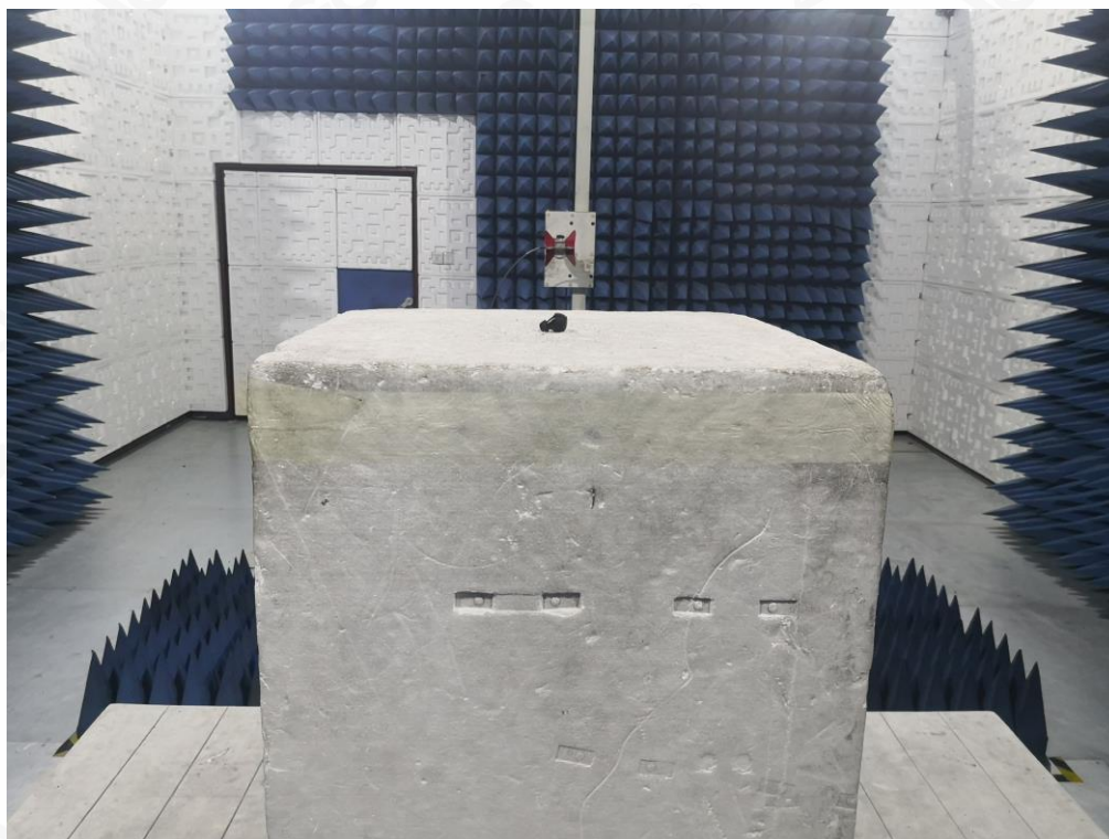
RADIATED EMISSION TEST SETUP ABOVE 1GHZ
