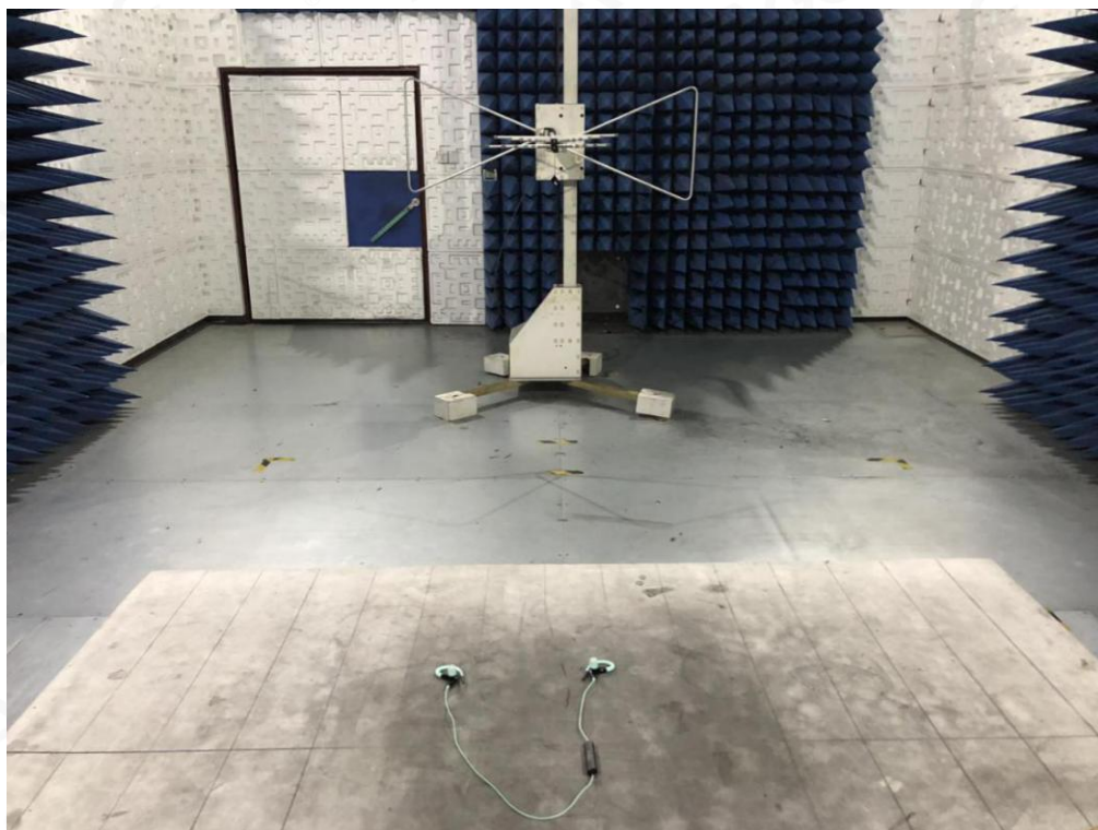
RADIATED EMISSION TEST SETUP ABOVE 1GHZ
