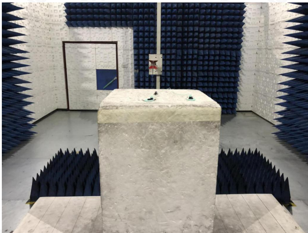
RADIATED EMISSION TEST SETUP ABOVE 1GHZ
