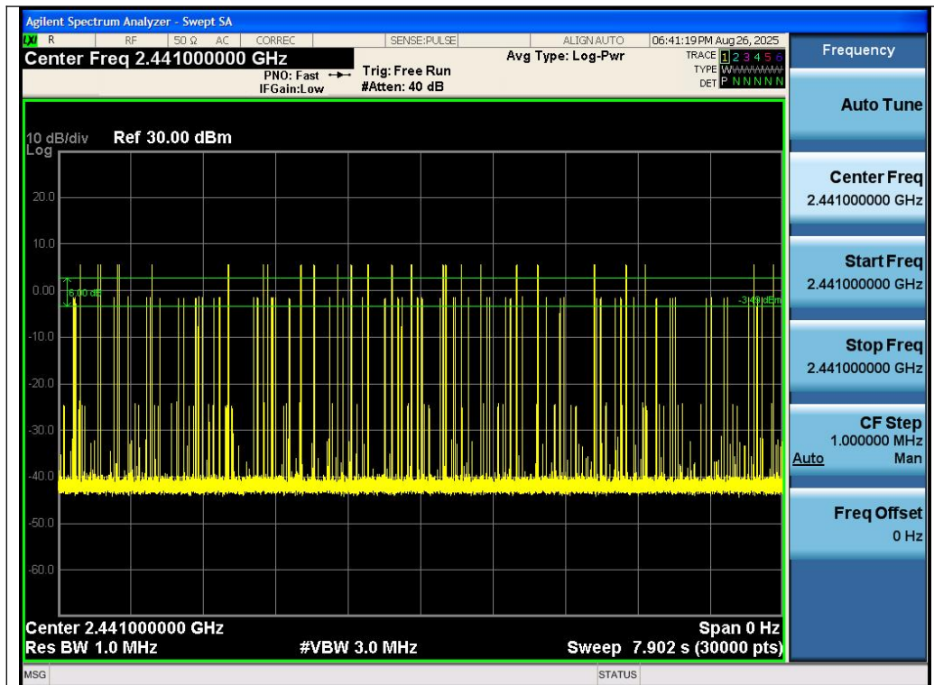
Test_Graph_BR_HOP_ANT1_NA_3Mbps_2441_Number of Busrt
