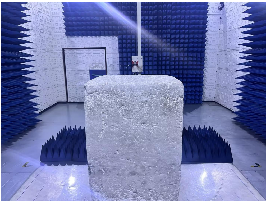
RADIATED EMISSION TEST SETUP ABOVE 1GHz
