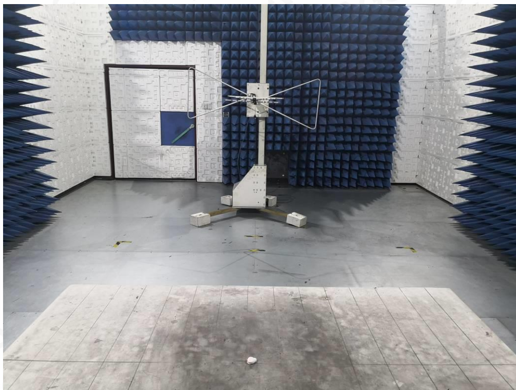
RADIATED EMISSION TEST SETUP ABOVE 1GHZ
