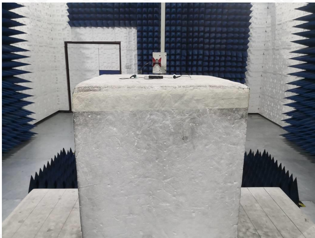
RADIATED EMISSION TEST SETUP ABOVE 1GHZ
