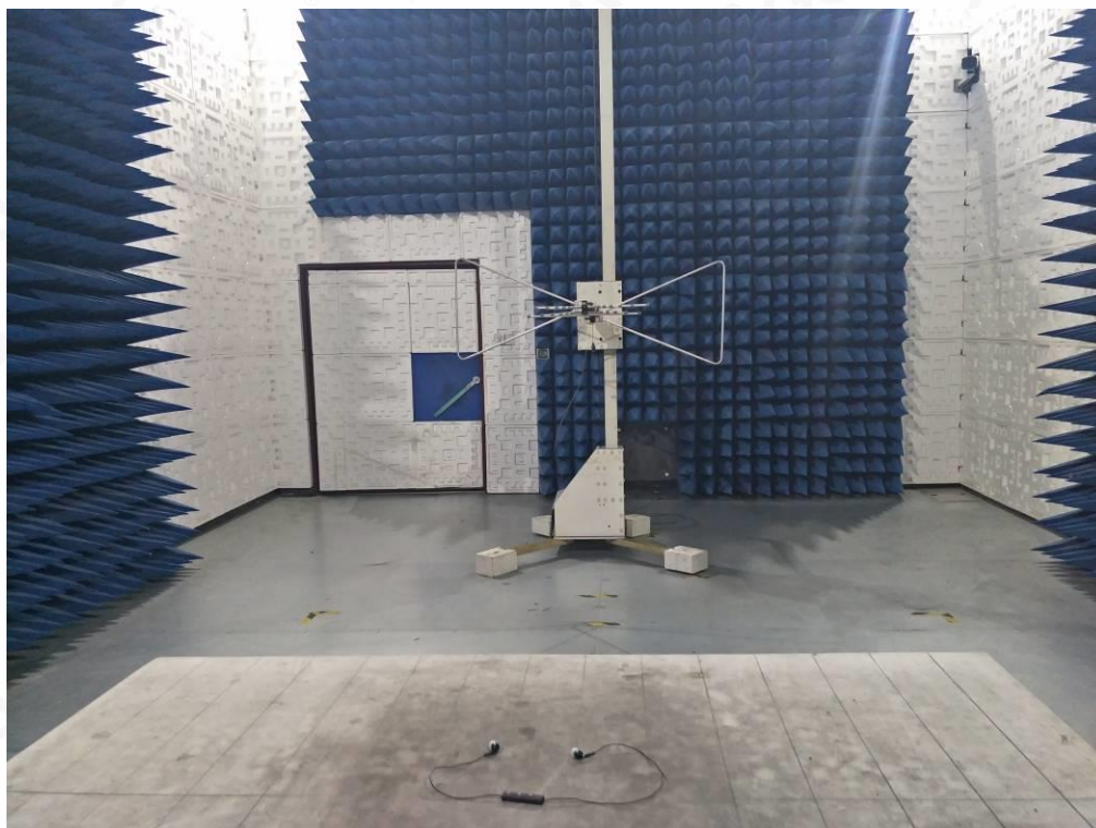
RADIATED EMISSION TEST SETUP ABOVE 1GHZ
