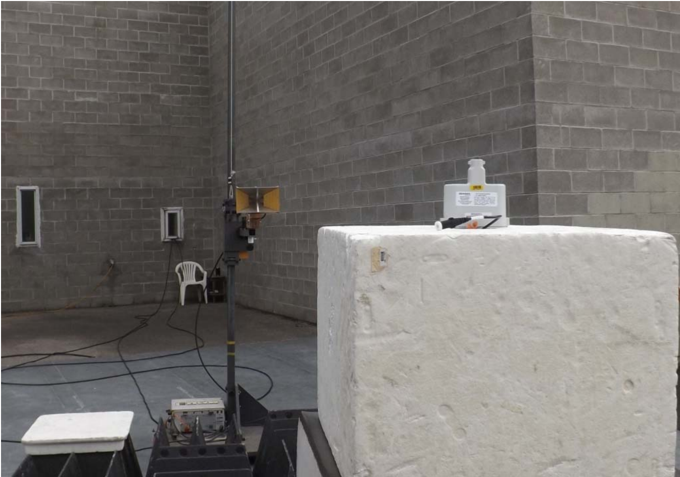
Figure E23.7 – Setup, Radiated Emissions, 1 – 10GHz, Vertical Polarization
