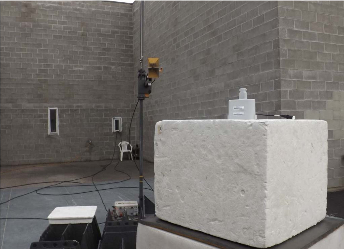
Figure E23.6 – Setup, Radiated Emissions, 1 – 10GHz, Horizontal Polarization
