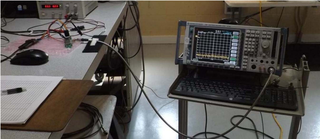
Figure E23.1 – Setup, Conducted Measurements
