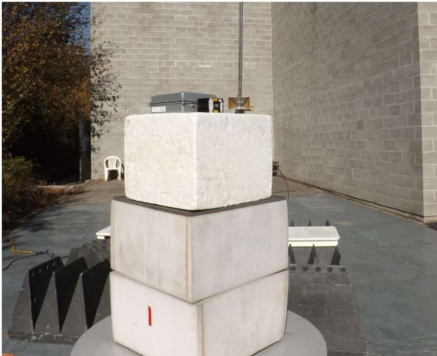
Figure E18.3 – Setup, Radiated Tx 1 - 10GHz
