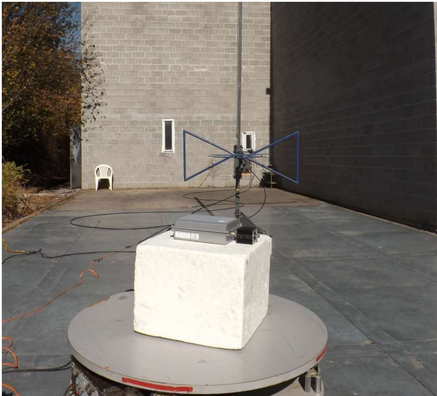
Figure E18.2 – Setup, Radiated Tx 30 - 1000MHz
