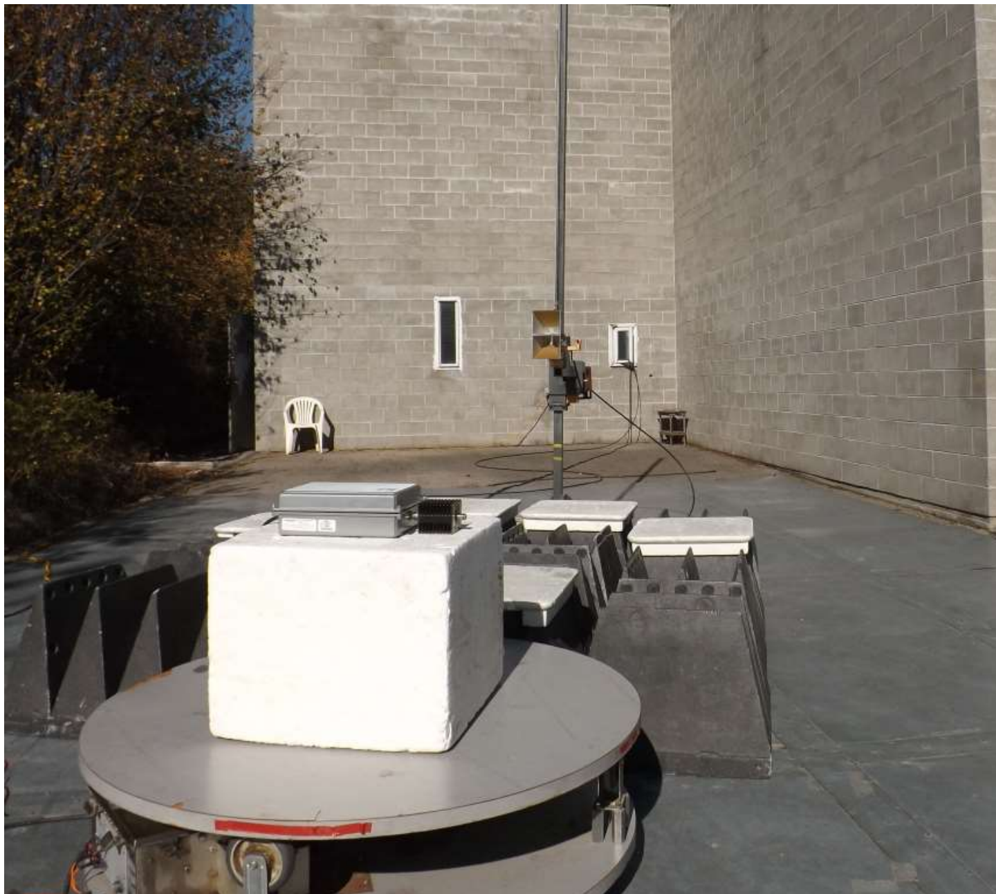
Figure E18.4 – Setup, Radiated Rx 1 - 10GHz
