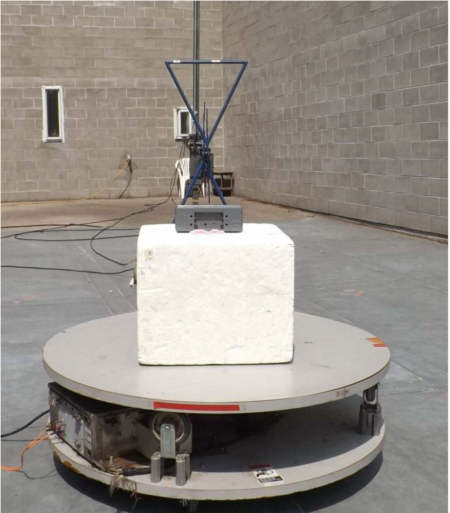
Figure E23.3 – Setup, Radiated Measurements, 30 - 1000MHz
