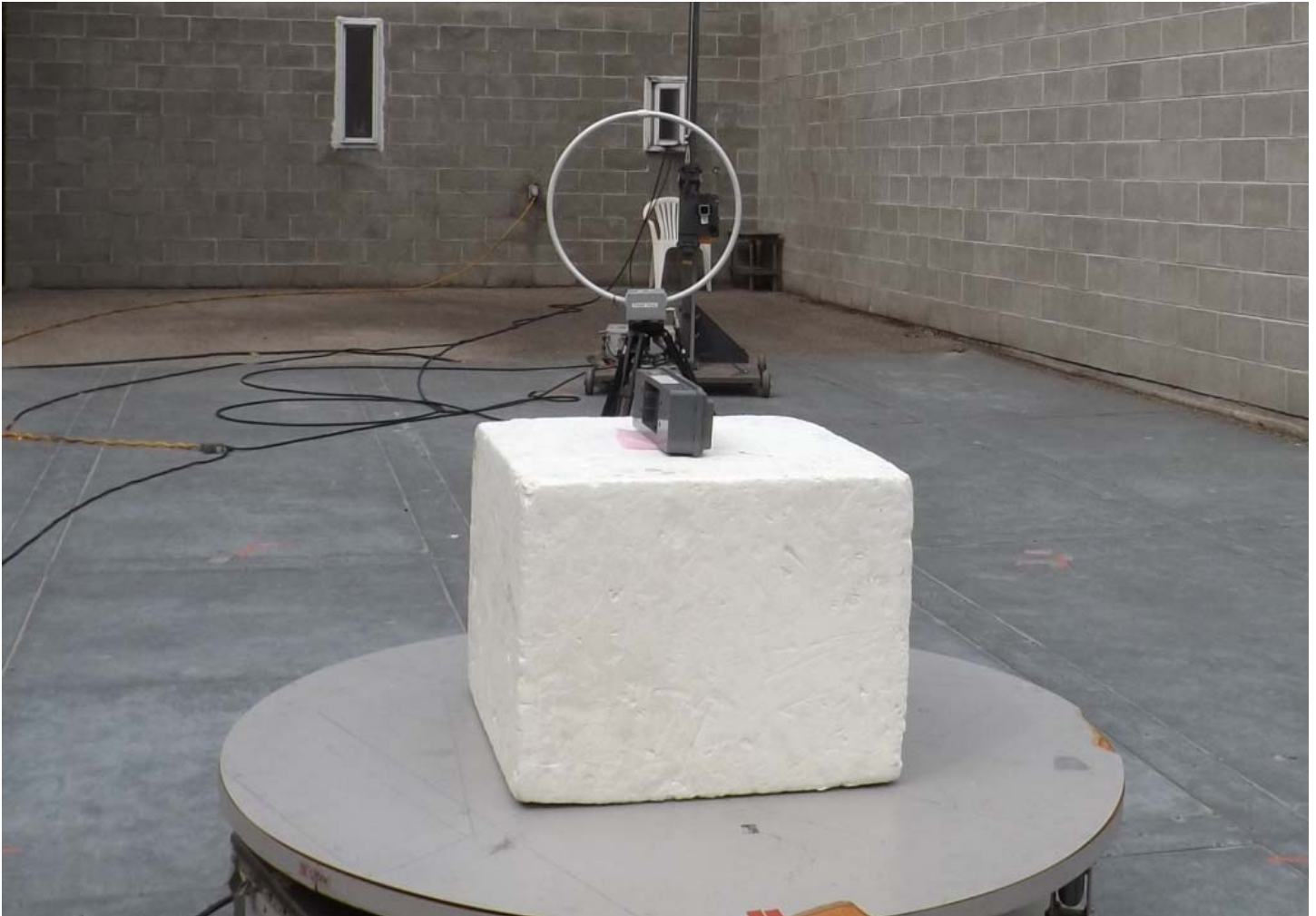
Figure E23.2 – Setup, Radiated Measurements, 9kHz – 30MHz
