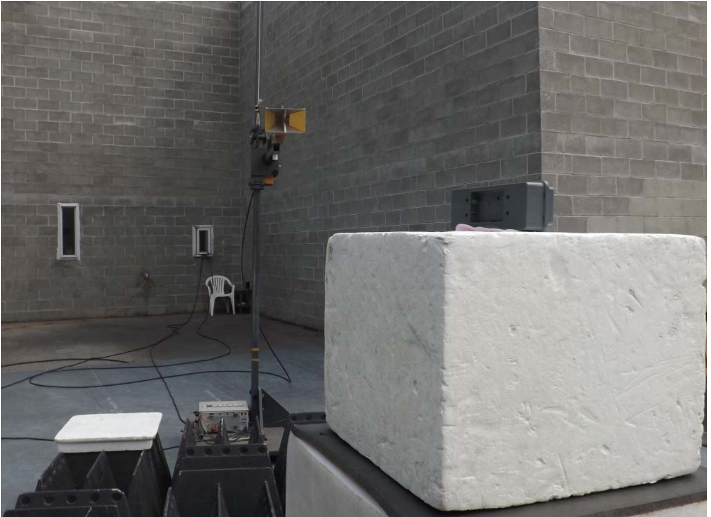
Figure E23.4 – Setup, Radiated Measurements, 1 – 18GHz
