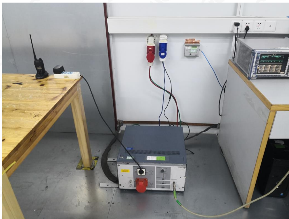
RADIATED EMISSION TEST SETUP-BELOW 1GHZ
