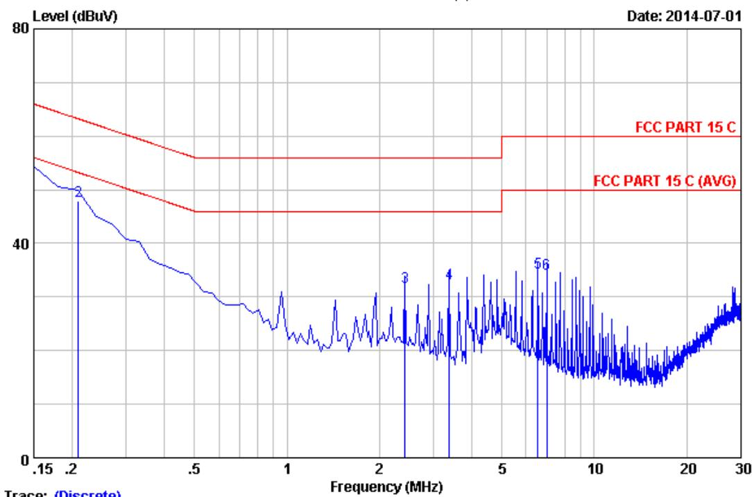
Remarks: 1. Emission Level=LISN Factor+Cable Loss (Include 10dB pulse limit)
