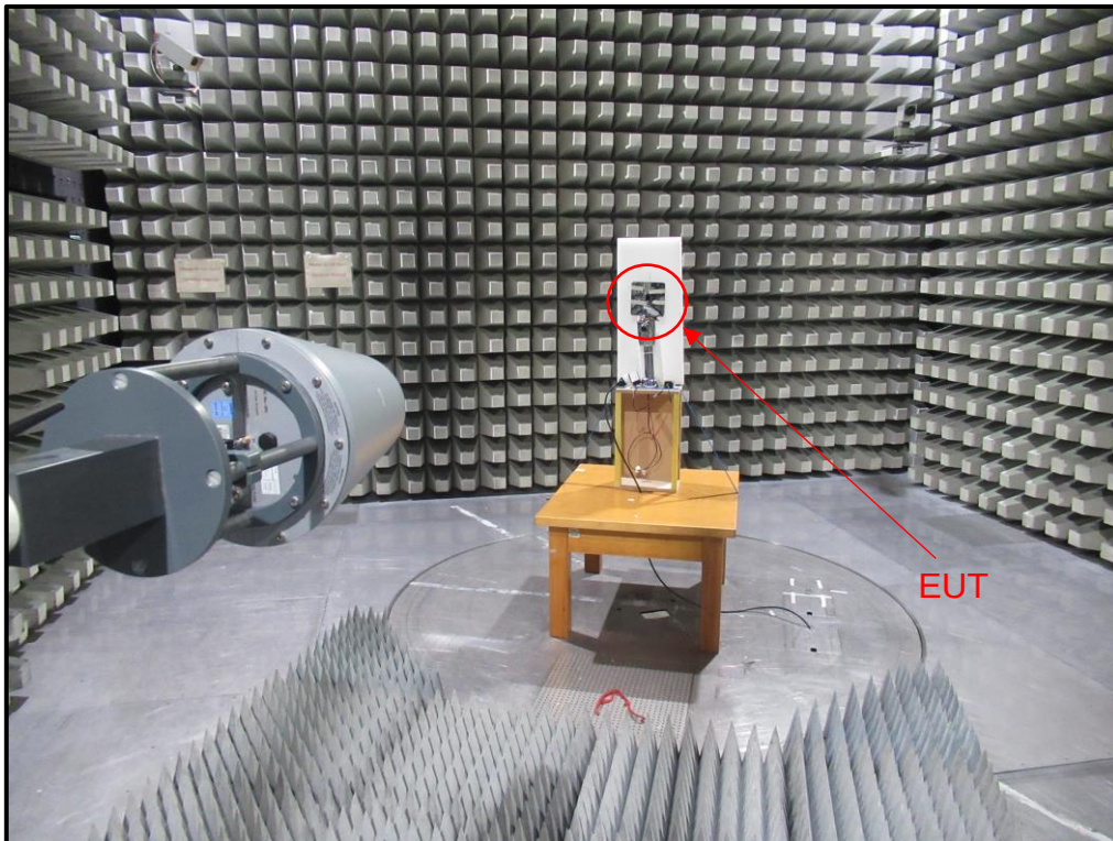
Photo 11: Radiated Test Setup - 1 GHz to 18 GHz - EUT+ PCB Antenna
