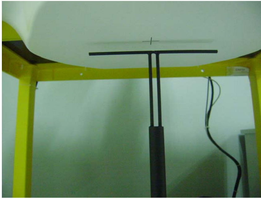
Setup Photo of Dipole Antenna
