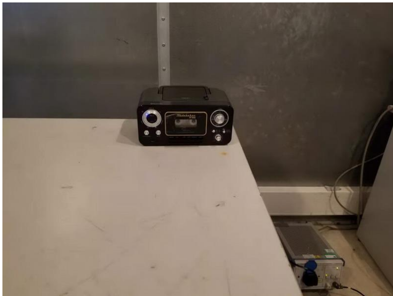
Measurement of Conducted Emission Test Set Up
