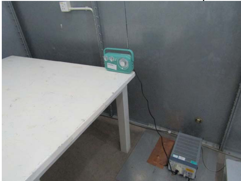
Measurement of Conducted Emission Test Set Up
