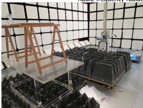
Unwanted emissions into Restricted Frequency Bands (18 GHz -26 GHz) and Unwanted emissions into non-Restricted Frequency Bands (1 GHz -25 GHz)
