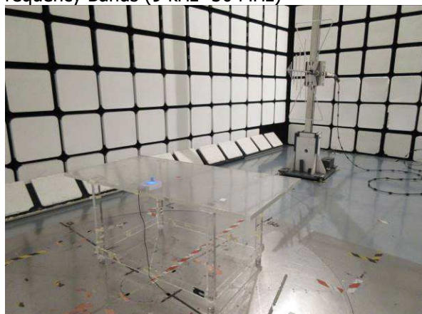
Unwanted emissions into Restricted Frequency Bands (30 MHz -1 GHz) and Unwanted emissions into non-Restricted Frequency Bands (30 MHz -1 GHz) and Radio-frequency radiated emissions (30 MHz – 1 GHz)
