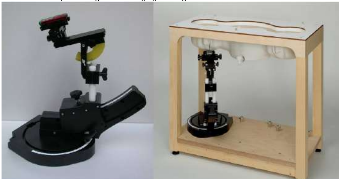
Device holder supplied by SPEAG
