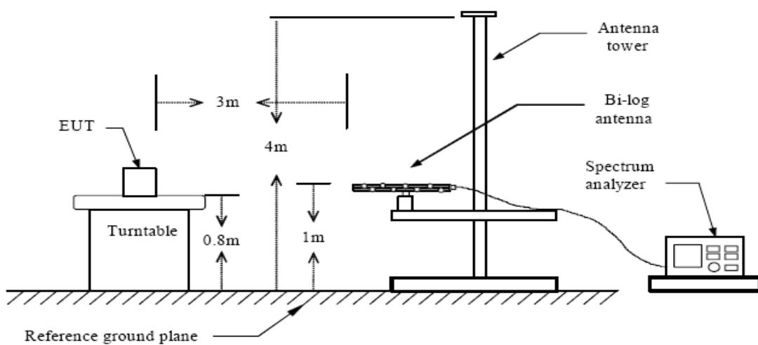
For radiated spurious emissions above 1GHz
