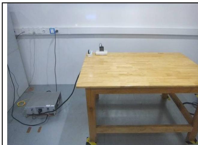
Conducted Emissions Test Setup Front View
