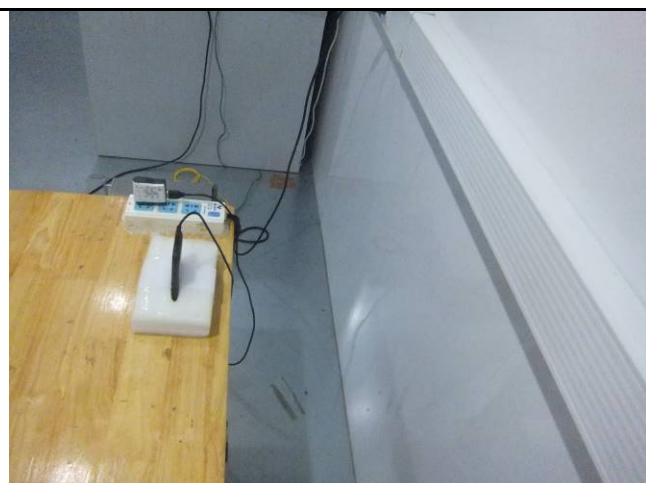
Conducted Emissions Test Setup Side View
