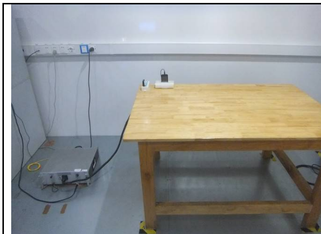
Conducted Emissions Test Setup Front View
