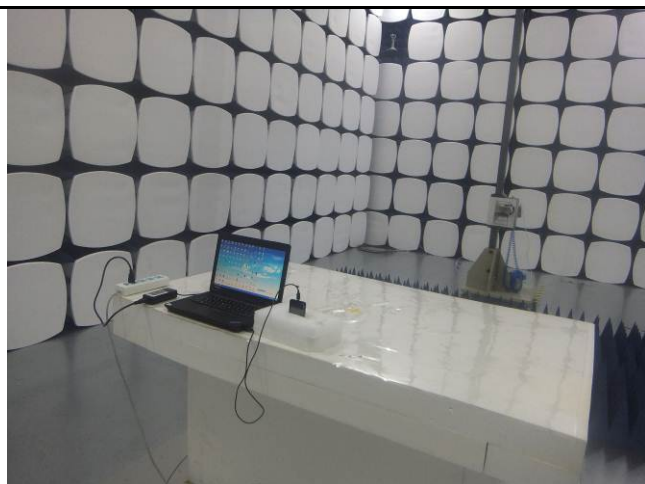
Radiated Spurious Emissions Test Setup Above 1GHz
