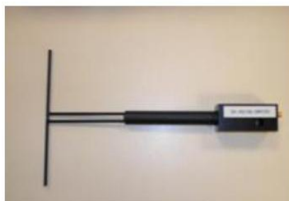
Figure 1 – Satimo COMOSAR Validation Dipole
