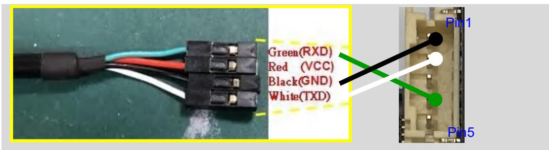
**Warning: Do NOT connect Red terminal (VCC) to Debug connector**
