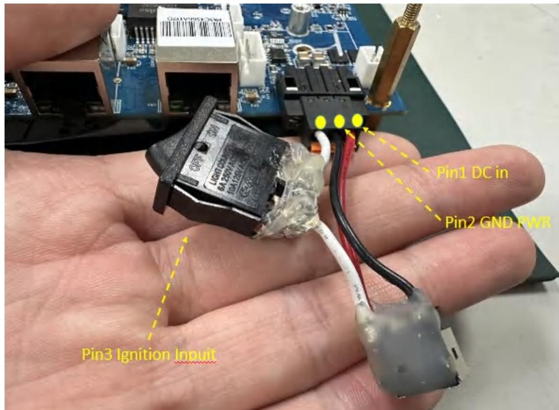
The MCU will always detect an ignition signal as long as DC adapter is on can be turned on SBC4100\_NSD4100.
