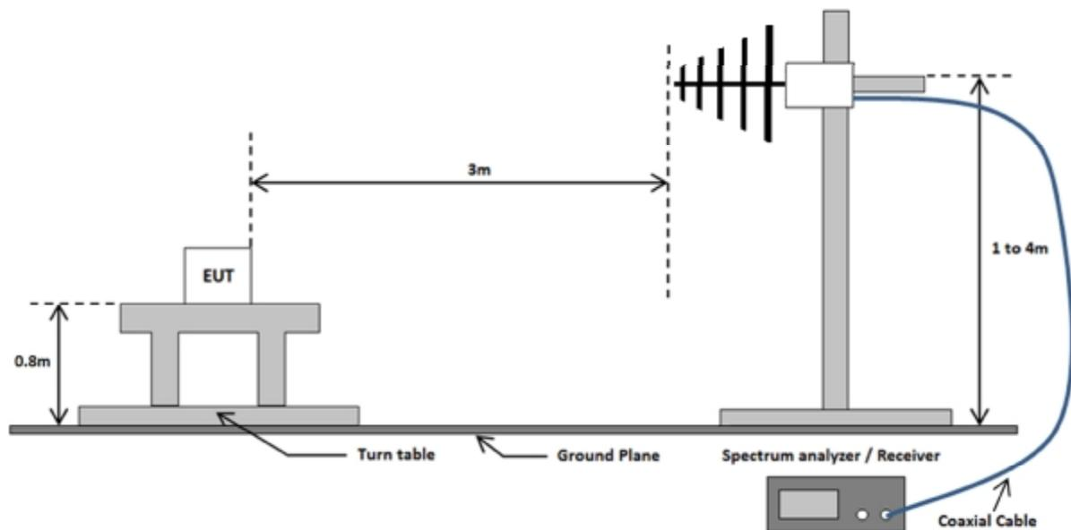
Radiated emissions test setup above 1 GHz
