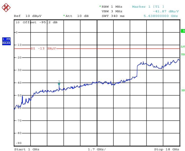
UE transmits at Band 2, channel 18900 with 10 MHz BW, antenna polarization is Vertical.
