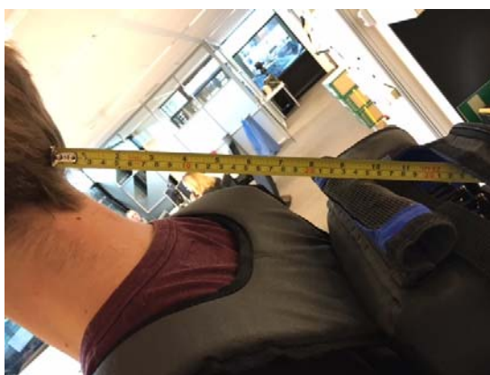
Figure 3: also insure that the distance between the antenna array and the head is bigger than 2.5 cm carying the AgileR in a backpack
