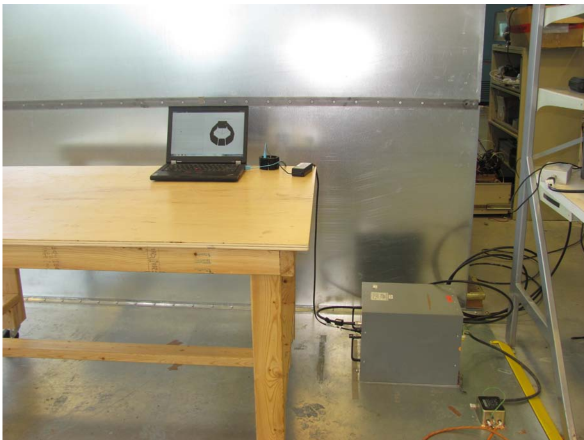
Illustration 7: Power line conducted emission setup – photo 1
