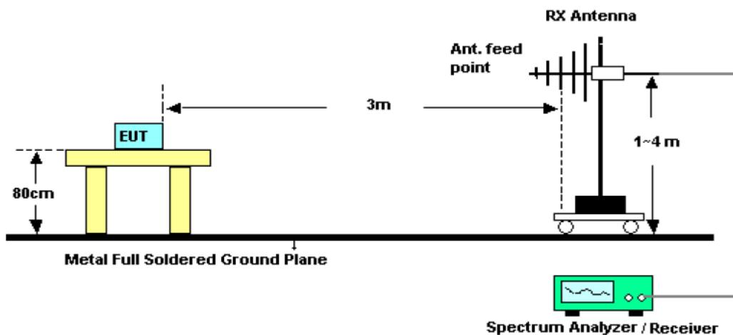
For radiated emission from above1GHz
