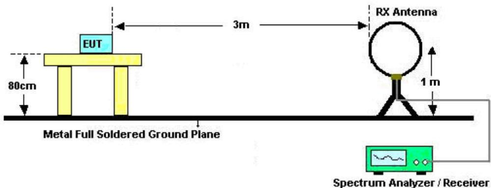
For radiated emission from 30MHz to1GHz
