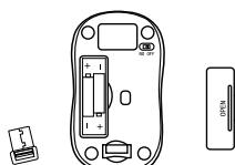
Open the battery compartment put two AAA battery into battery compartment, insert the battery as shown inside the battery compartment.
