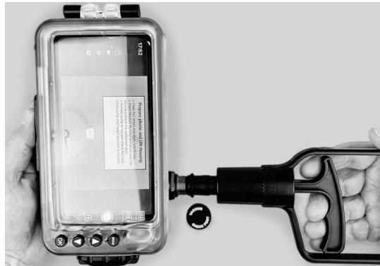
Hand pump pressed against vacuum check port
