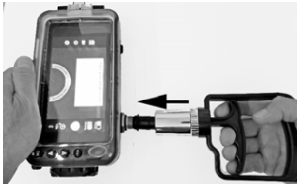
Hand pump pressed against vacuum check port
