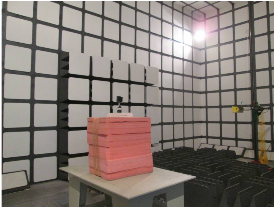
Transmitting Radiated Emissions View (Above 1 GHz)
