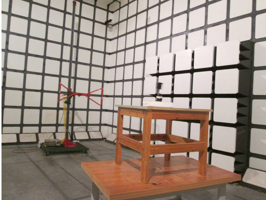
Transmitting Radiated Emissions View (Below 1 GHz)
