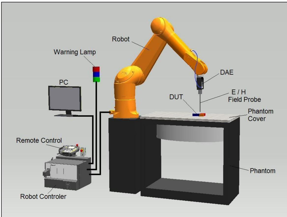
The DASY5 system for performing compliance tests consists of the following items:
