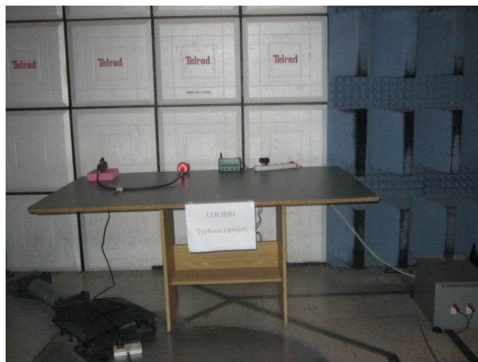
Figure 2. Conducted Emission Test
