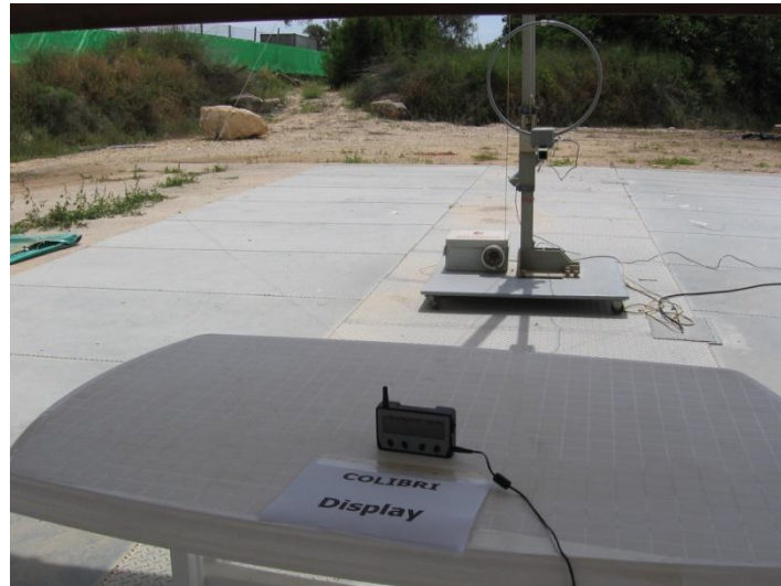
Figure 4. Radiated Emission Test
