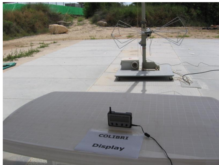
Figure 5. Radiated Emission Test
