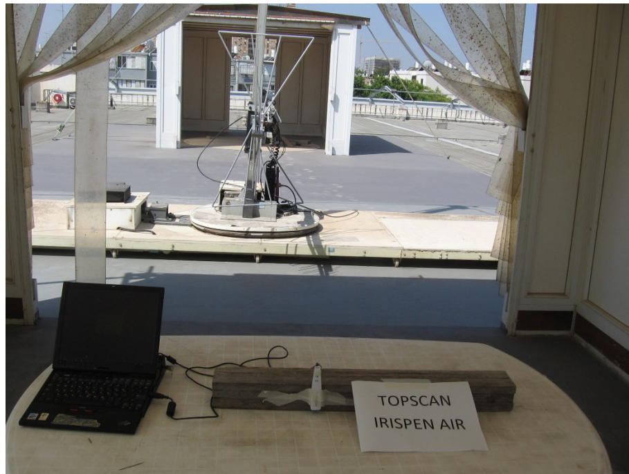
Figure 5. Radiated Emission Test
