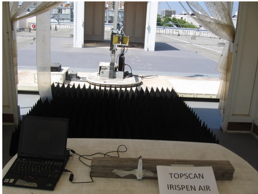
Figure 6. Radiated Emission Test
