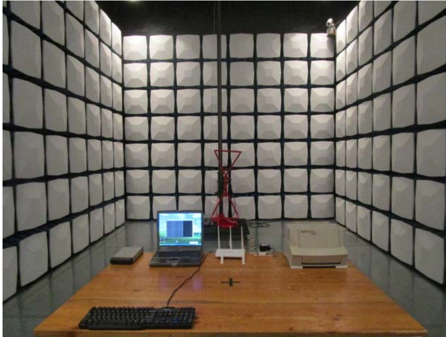
Radiated Emission Below 1GHz –Front View
