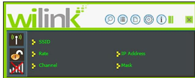
The function buttons on the top (From L to R) are: Available Networks, Link Information, Profile Settings, Advanced, and About. While the left column displays Turn On/Off RF, Security /No security, and Signal status.
