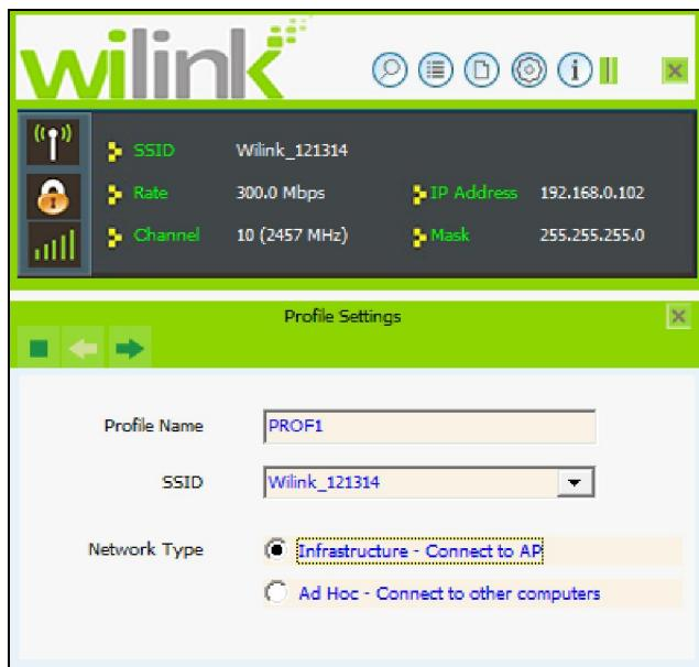
Infrastructure is an application mode that integrates the wired and wireless LAN architectures. It is different from Ad-Hoc in that in this mode the computer installed with the wireless network adapter has to fulfill the wireless communication via AP or wireless router. It can be divided into two modes: wireless AP + wireless network adapter and wireless router + wireless network adapter.
