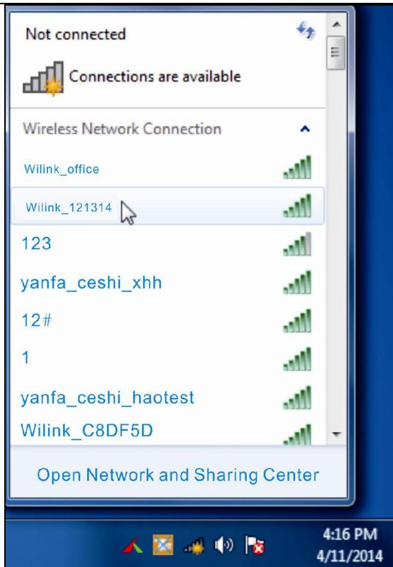
When the highlighted part shows **Connected**, the connection is successful.
