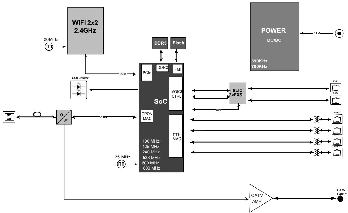
Figure 2.1-1: ONT-RGWRF circuit block diagram
