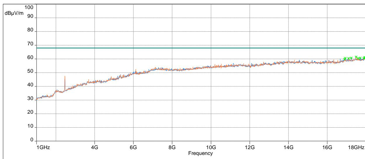
Radiated Spurious Emissions 1000 - 18000 MHz, Avg Scan vs Avg Limit
