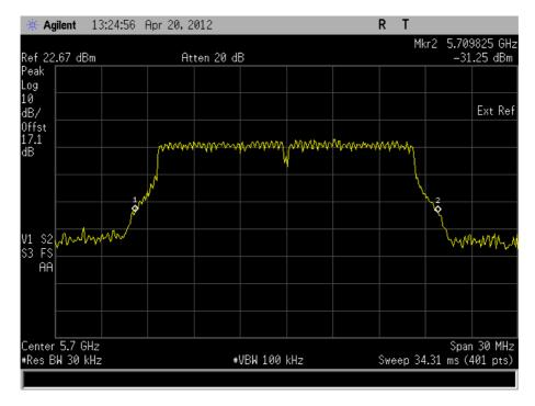
The test was performed on the worst case data rate for 802.11(a) modulation. The worst case was deemed as the data rate which produced the highest level of conducted average power. This data rate was 54Mbps.
