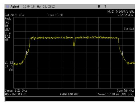
The test was performed on the worst case data rate for 802.11(n) - 40 MHz BW modulation. The worst case was deemed as the data rate which produced the highest level of conducted average power. This data rate was 135Mbps.
