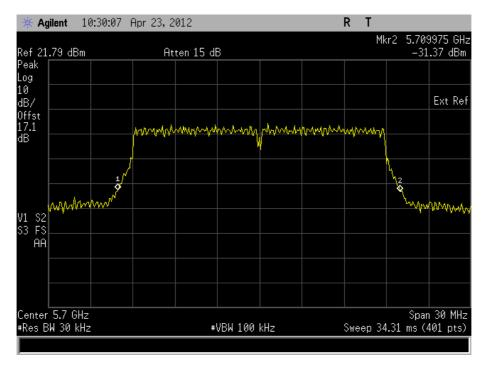
The test was performed on the worst case data rate for 802.11(n) - 20 MHz BW modulation. The worst case was deemed as the data rate which produced the highest level of conducted average power. This data rate was 21.70 Mbps.
