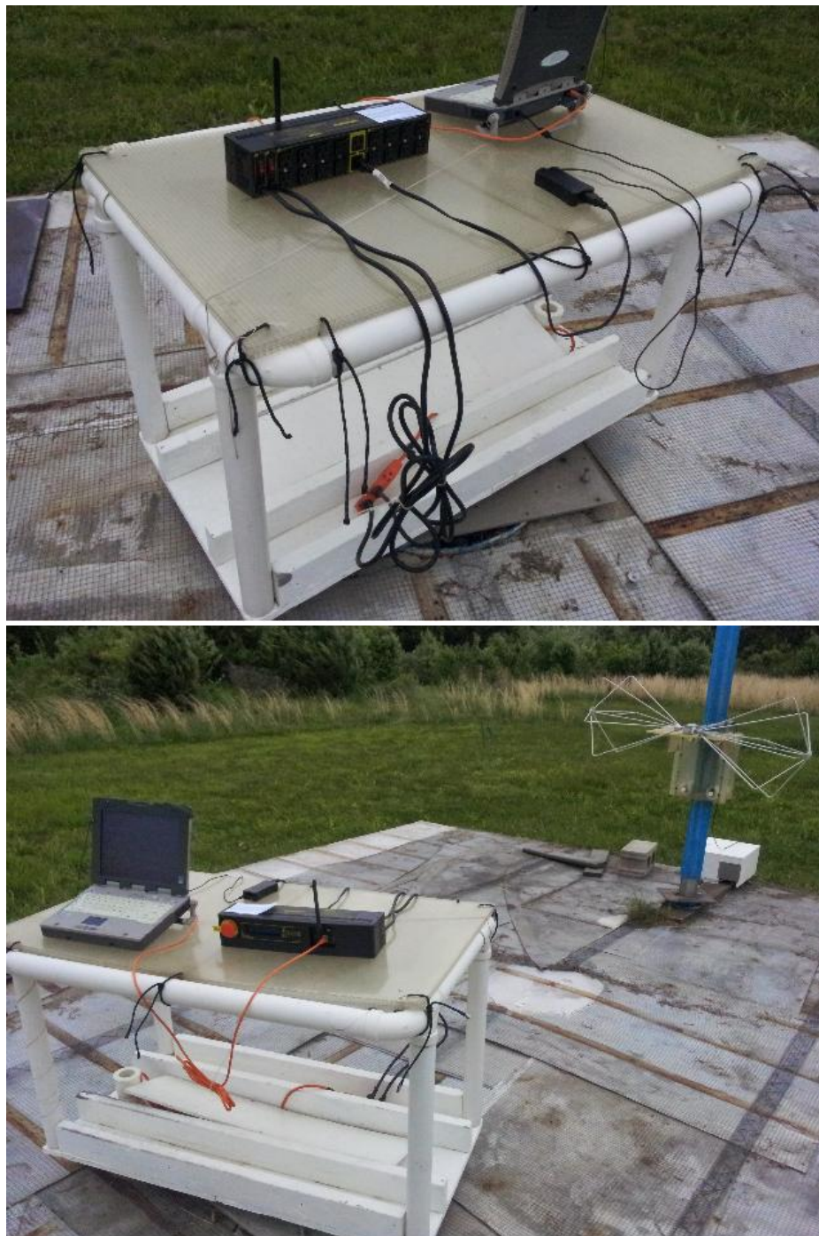
Figure 4: Radiated Emissions Test Setup Photograph(s).
