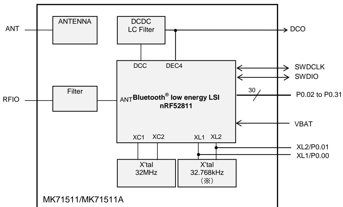
(※) MK71511A does not built-in a 32.768kHz crystal oscillator.
