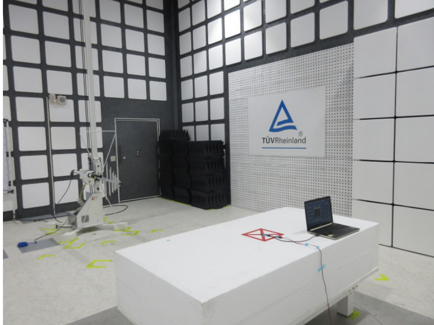
Photograph 4: Set-up for Spurious Emissions (Back View 2)
