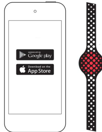
Click on the core to check the battery level. The battery is charged if the light is blinking.
