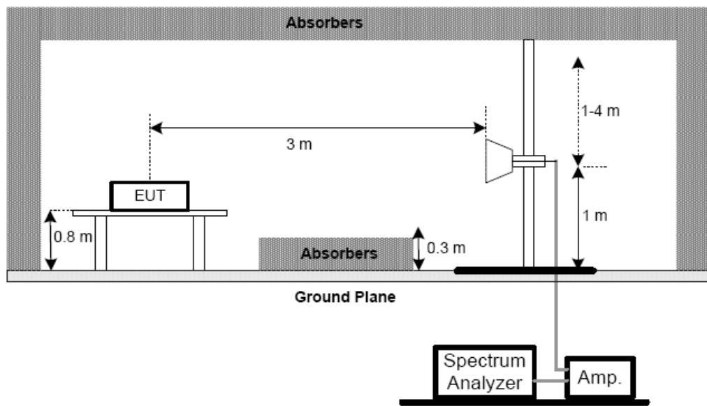
(C) For radiated emissions below 30MHz
