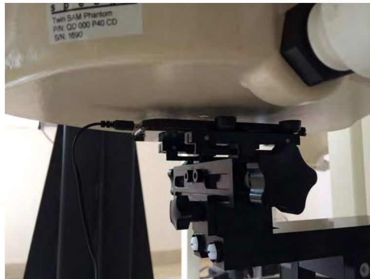
10mm Body-worn Rear(with Headset) Setup Photo
