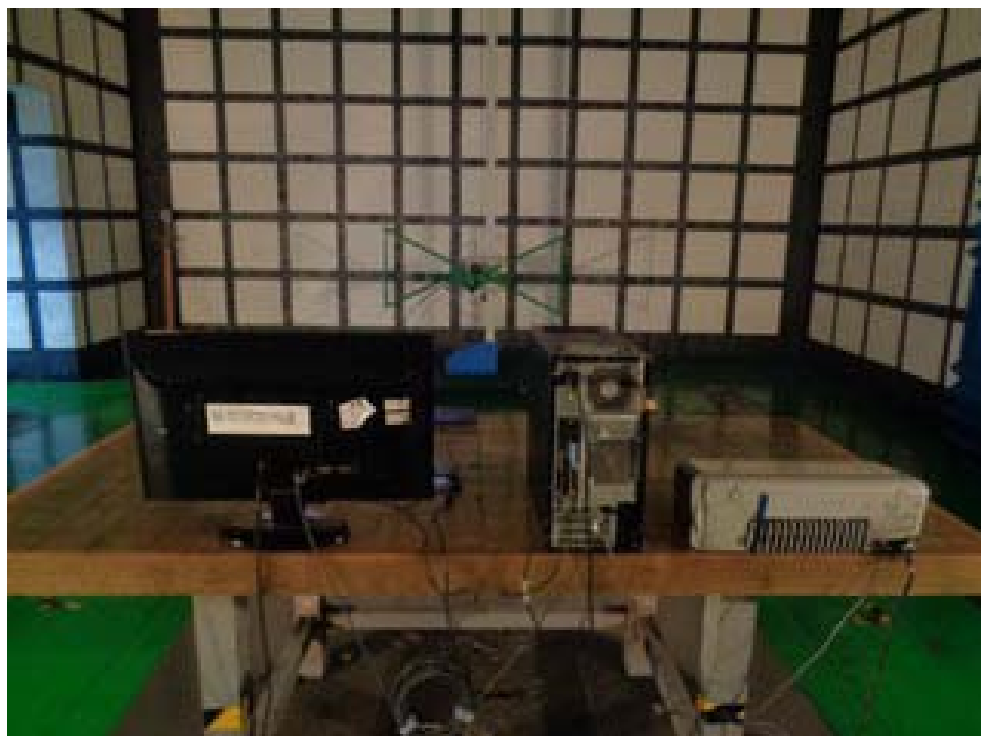
Photograph 4: Radiated Emission Test Configuration, (Below 1GHz) Back
