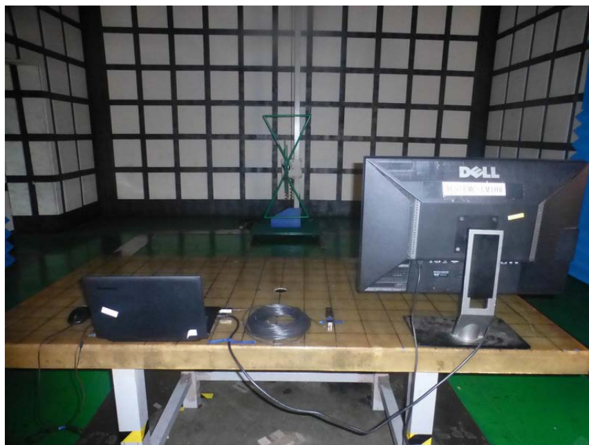
Photograph 4: Radiated Emission Test Configuration, (Below 1GHz) Back
