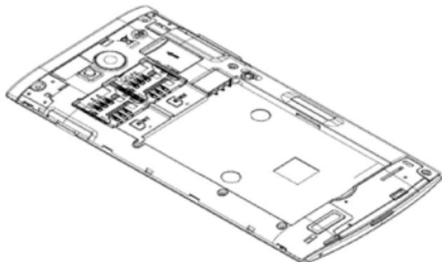
4. Insert the battery by aligning the gold contacts on the battery with the gold contacts in the battery compartment. Gently push down on the battery until it clicks into place.
