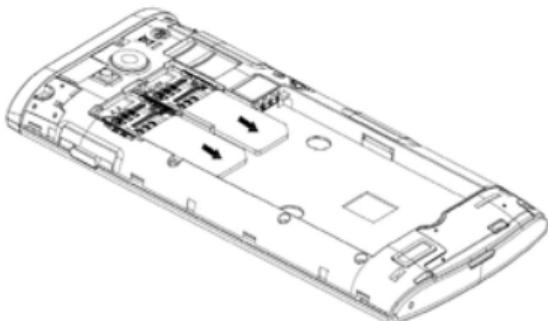
3. Insert the memory card into the metal slot with the metal contacts facing down until it clicks to the right position.]
